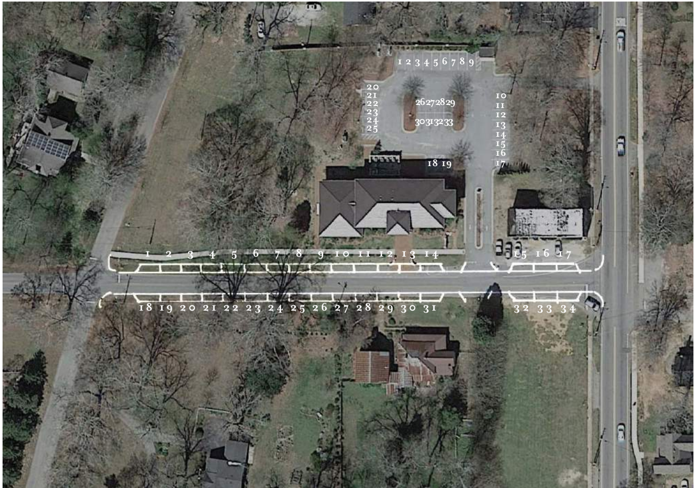
Aerial view of West Clark St. comparing existing off-street parking lot spaces at City Hall to the number of parallel parking spaces that could be accommodated on street.
